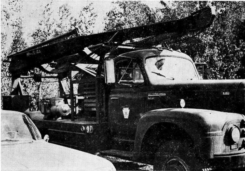
SPECIAL HOIST RIG —Pennsylvania Department of Mines truck containing special hoisting rig stands ready to aid in pulling entombed miners from their underground chamber.
